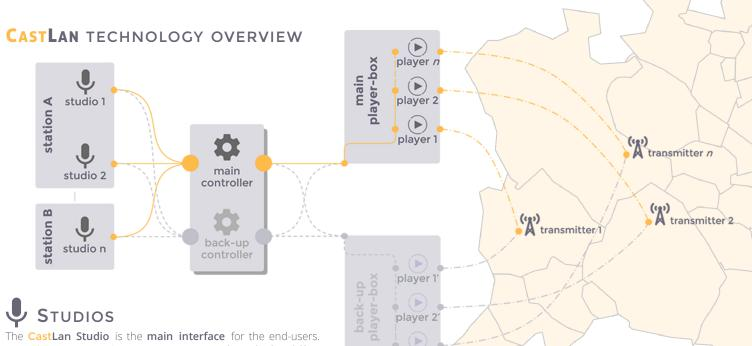
From this one, manual or automatic triggers launch the different breaks of the loaded playlist. Furthermore, it allows to take control over some or all the transmitters of a dedicated station, such that they are linked to the appropriate studio at the right time.
